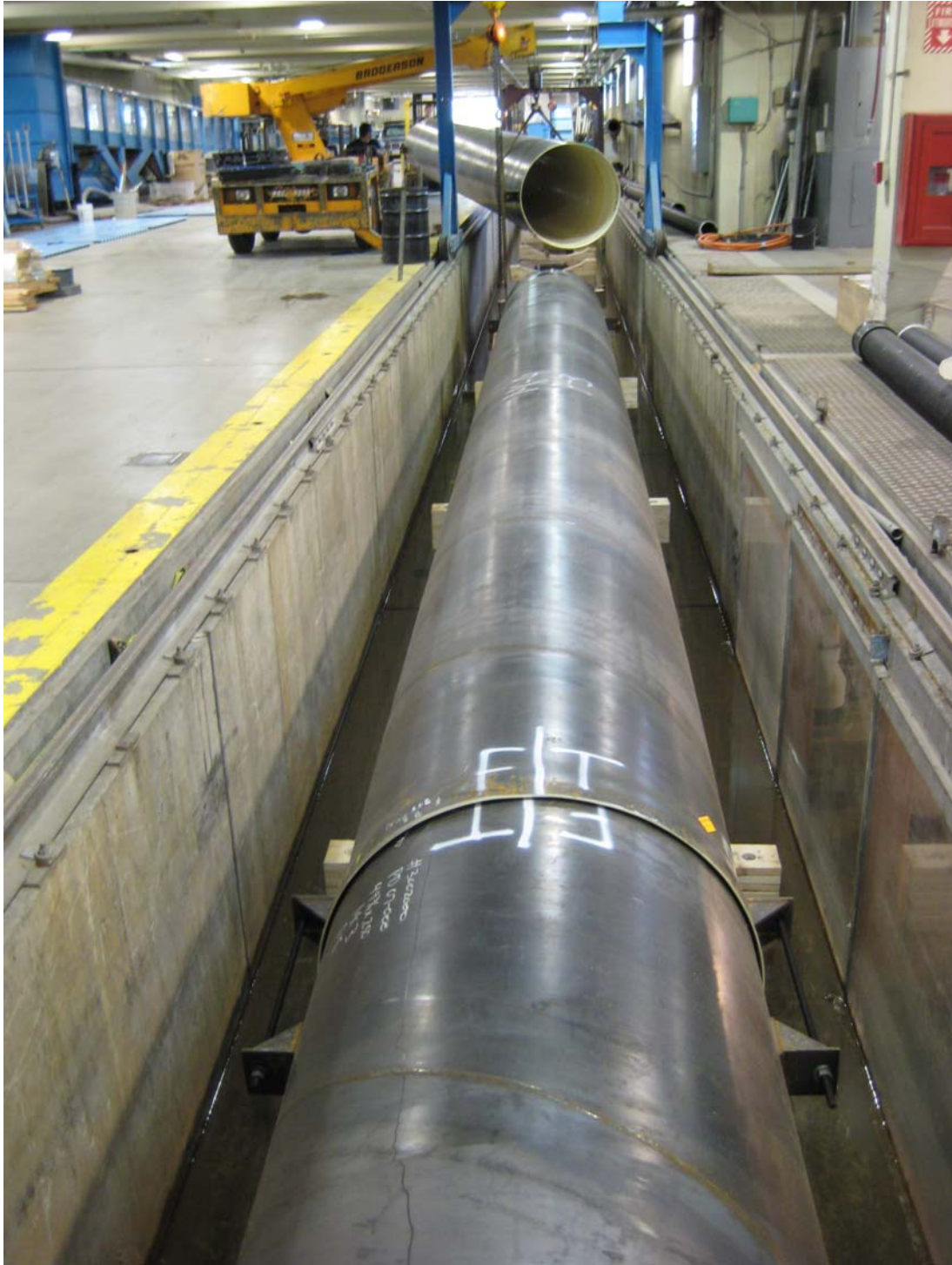
Figure 1. Installation of 48-inch Polyurethane-Lined Steel Pipe Test Setup
